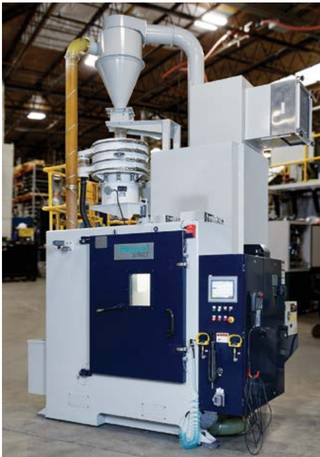
A Progressive Surface robotic Shot Peen System will be installed in Purdue University's Materials and Manufacturing Research Laboratory.
