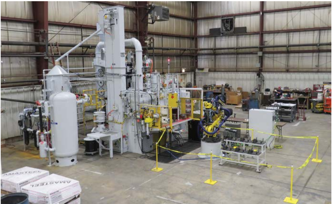
72" Flex Peener three (3) Spindles at each Station for High Volume Gears. Can do Eight (8) Different Type Gears with our Patent Pending one pc. Tooling Holders. Shown with Robot Load.
