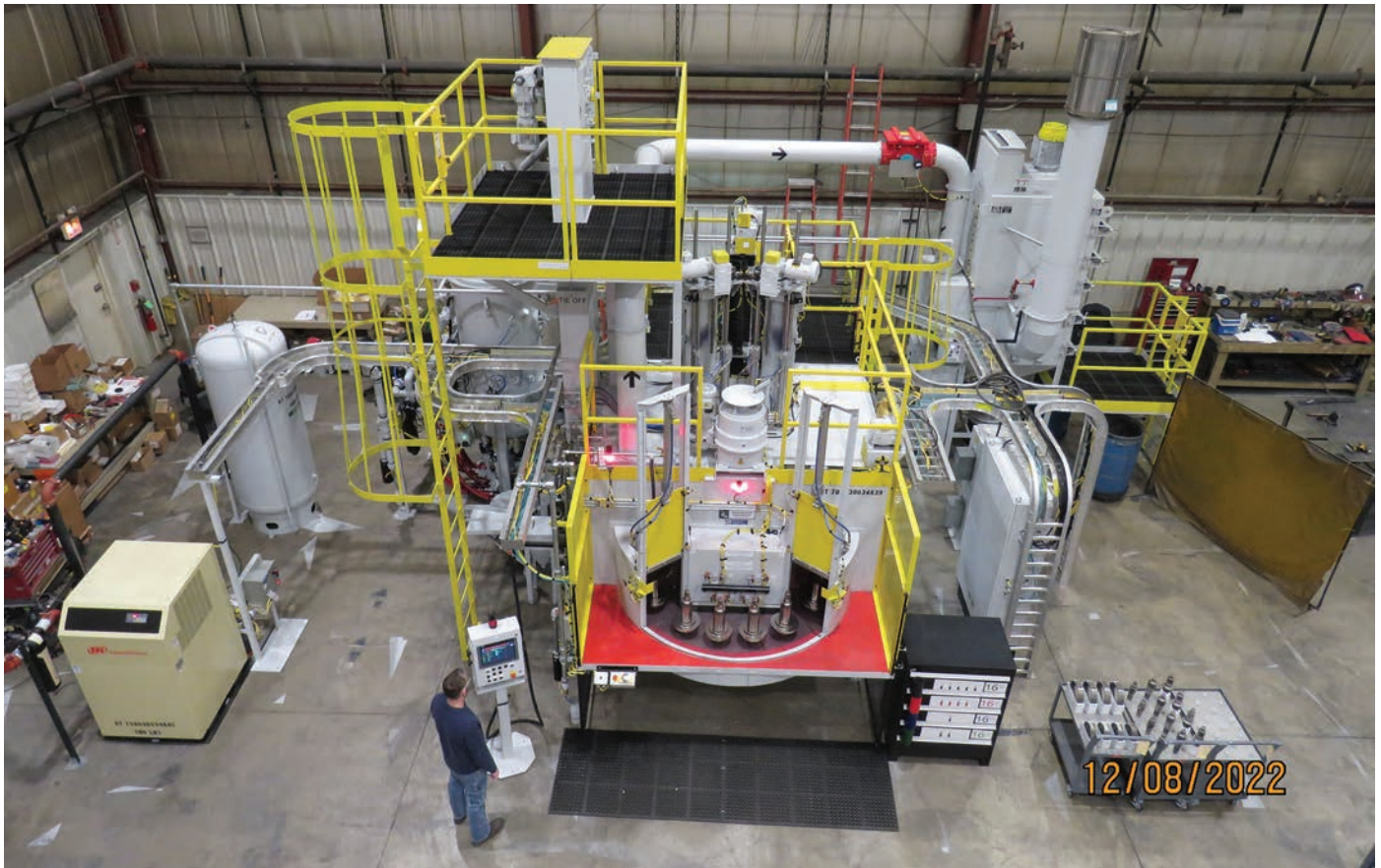
84" Flex Peener Four (4) Spindles at each Station for High-Volume Gears. Can do Eight (8) Different Type Gears with our Patent Pending one pc. Tooling with Robot Load.
