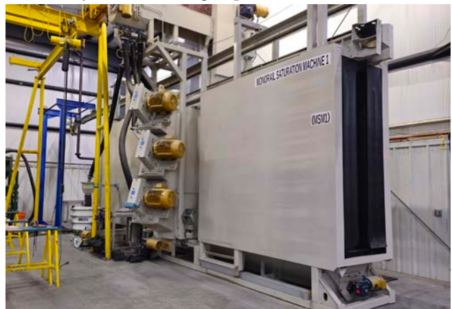
Figure 1. Automated wheel-type shot-peening cell for large aerospace components.
