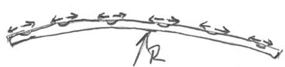
Figure 2 - Convex Bending of the Almen Strip at the Peened Surface
