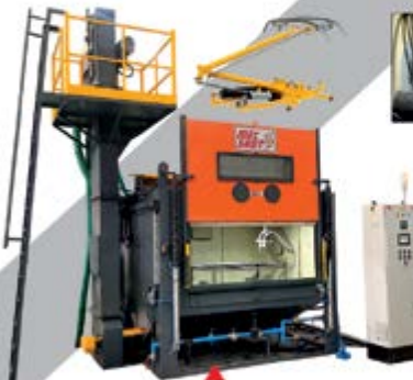
Spl. Blasting M/C for Roof-Mounted Pantographs Contact Strip Of Electric Rails & Tramways
