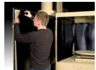
Figure 2. Rubber curtains extend cabinet life by protecting interior walls from blast media.
