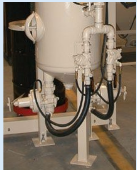
Figure 3. Supplying six blast guns is relatively straightforward as demonstrated by the single air manifold and media hopper, each with six hose outlets.
