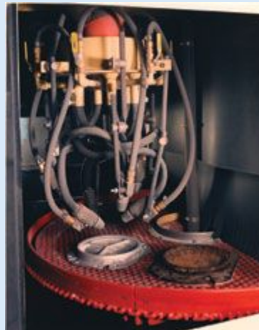
Figure 2. Besides simplifying piping to multiple blast outlets, suction systems make possible innovations like the rotary blast head. Equipped with six blast guns, the head shown spins to provide even coverage on broad work surfaces.
