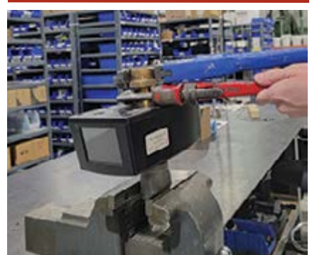
A how-to tip when attaching or removing pipe fittings: Use two pipe wrenches—one on the valve pipe and one on the pipe fitting.
